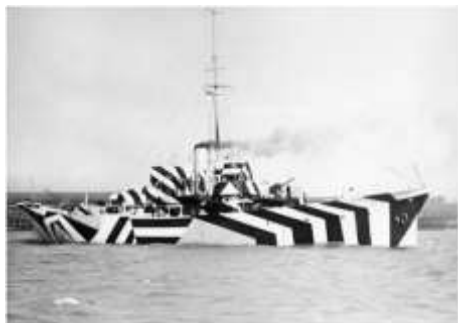
HMS Kildangan, sister ship of HMS Kildorrey in 'dazzle' camouflage (designed to break up the outline of the ship as seen through a submarine's periscope). IWM via Wikipedia
